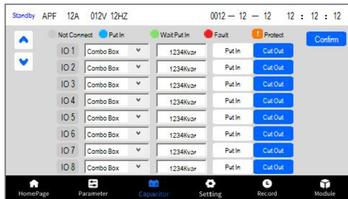
Figure 4.7 Capacitor Switching Interface Second Page
